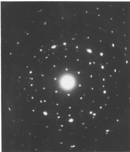
Figure 6 Electron diffraction pattern of a region of the sample shown in Fig. 2 containing only intergranular precipitates (triangular platelets).
